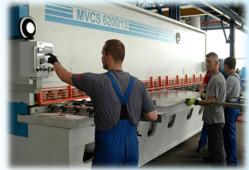
MVCS 6200/13 Jelšingrad Max cutting length 6.000 mm Max material thickness 13 mm
