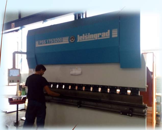
PSS 175/3200 Jelšingrad Bending 3.200 mm -175 tons
