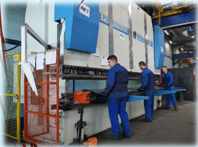
PSS 400/6000 Jelšingrad Bending 6.000mm- 400 tons
